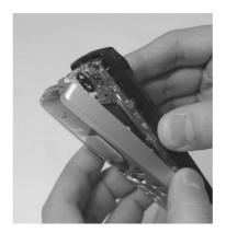
To remove the PWB from the housing, remove the seven screws.
