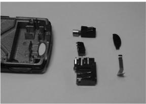
When taking the PWB and LCD module apart, remember the fixings on both sides of the LCD.
