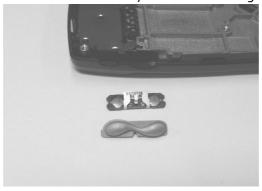
Remove the battery connector from its housing, using the SRT-3 tool.
