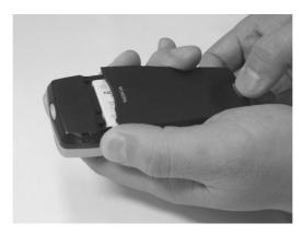
Lift the battery first from the bottom end.
