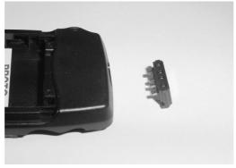
Remove the antenna by releasing the snap fixing on both sides of the phone.
